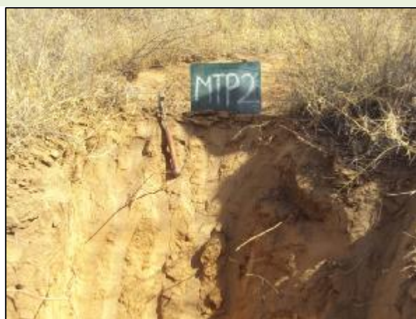
Figure 3: Typical test pit investigated on site (shallow refusal)
